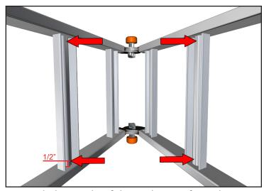
6. Mark the inside of the 2nd rungs from the top, 1/2" in from the rail on each side, along the centerline. Note: If straps were already riveted here, skip to step 8. Repeat steps 2-4 on remaining strap rivets.
