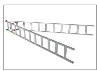
2. Lay the inner section on its side and open enough to access the strap rivets.
