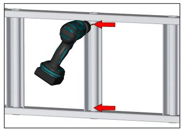
7. Using a 3/16" bit, drill new holes through the center of the rungs where marked. Be careful to only drill through the inner wall of the rung.
