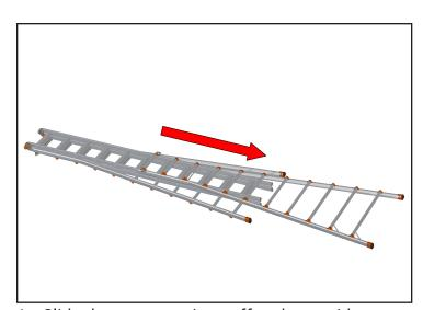
1. Slide the outer sections off and set aside.
