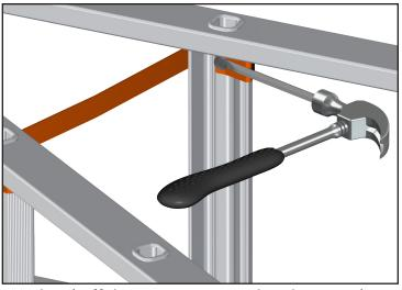
4. Chisel off the remaining rivet head material.
