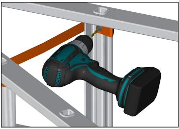
3. Using a 3/16" bit, drill through the center of the rivet head securing the straps. Do not drill past the rivet head.
