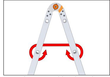
8. Wrap the straps around the 2nd rungs down from top to bottom.
