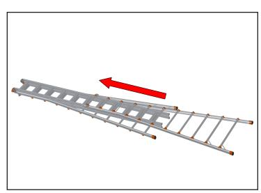
10. Slide the outer sections back on.
