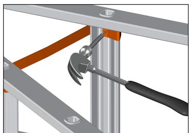
5. Tap the rivet out of the rung with a 3/16" punch.
